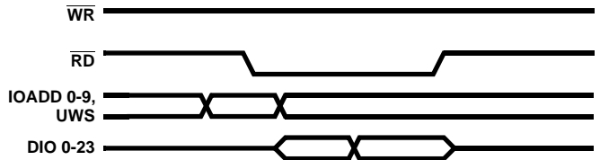
FIGURE 15. ASYNCHRONOUS 16/24 MODE TIMING
